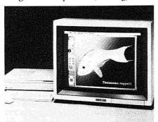
television-type signals, is compatible with IBM VGA and EGA/CGA, and runs with an IBM PC or compatible, or with the Macintosh II. That means that the trainer can connect it to many popular standard graphics controllers or any NTSC device, including a VCR or laserdisc player.
