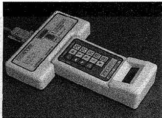
Completed test answers from keypads are downloaded to docking station.
