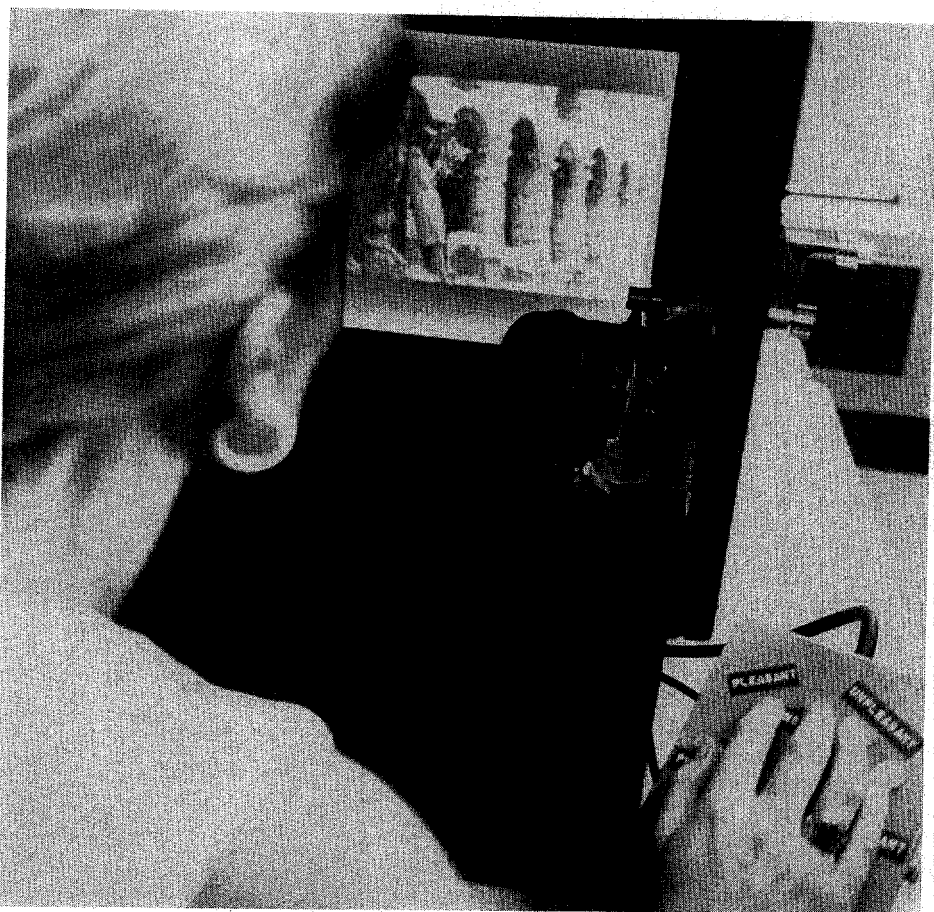
Measuring Reactions. Experiment subject shown above looks at projected pictures and pushes coded buttons to record her reactions. These reactions are then compared with a record of her pulse rate and pictures of her eyes, made by the camera in right foreground.
