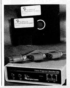
Hooked into a computer, it can control up to three projectors by itself, or up to 48 when linked with other Magician units. It can store up to 2,000 special effects at a time and go through them in sequence when the user presses the forward button on a standard remote cable. When the user holds the button for one-and-a-half seconds, the Magician automatically goes through all the effects stored in the computer memory, providing continuous operation for as long as the user wants.
