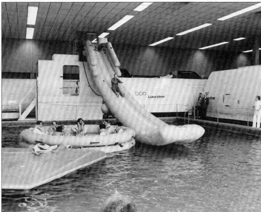
Cabin mock-ups give students an opportunity to experience the operation and use of emergency equipment firsthand.
