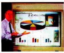
SoftBoard's electronic pen writes and draws in "electronic ink" on the product's surface. SoftBoard tracks the location of the pen using a laser scanning system; the projection-driver software coordinates the pen's position.
