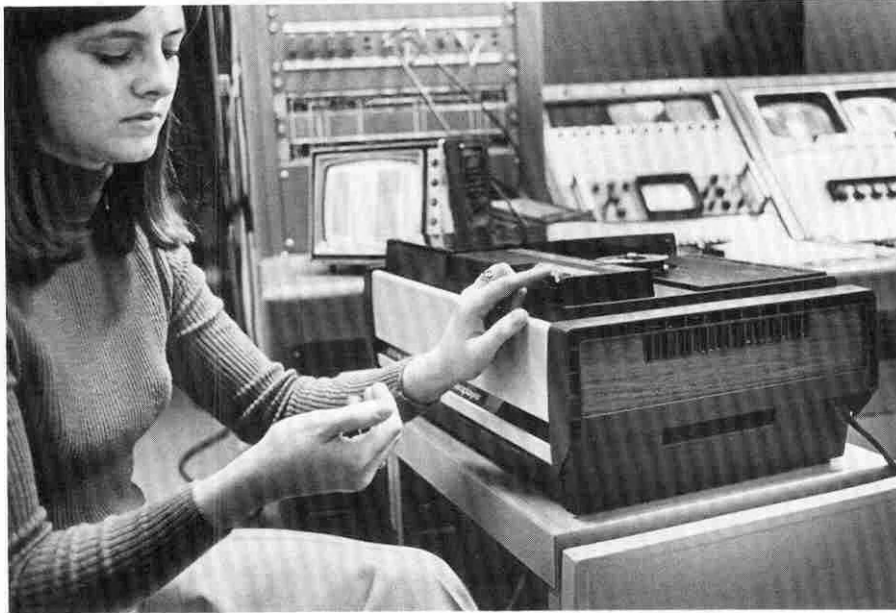
A simple stopwatch can be used to help manually synchronize the film video-player and videotape recorder during the film to tape transfer. It is simpler and faster than tape-to-tape editing using helical machines.
