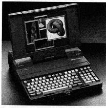
The 18.7-pound T5200 portable computer is designed for high-end desktop performance, and is available in two models—one with a 40MB and the other with a 100MB hard drive. Both feature, among other things,
